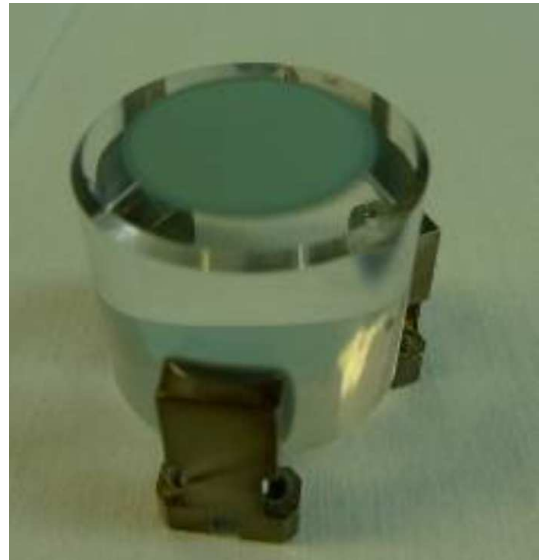
Fig. 5. Picture of the HRI EUV secondary mirror flight model before integration in the EUI instrument.
