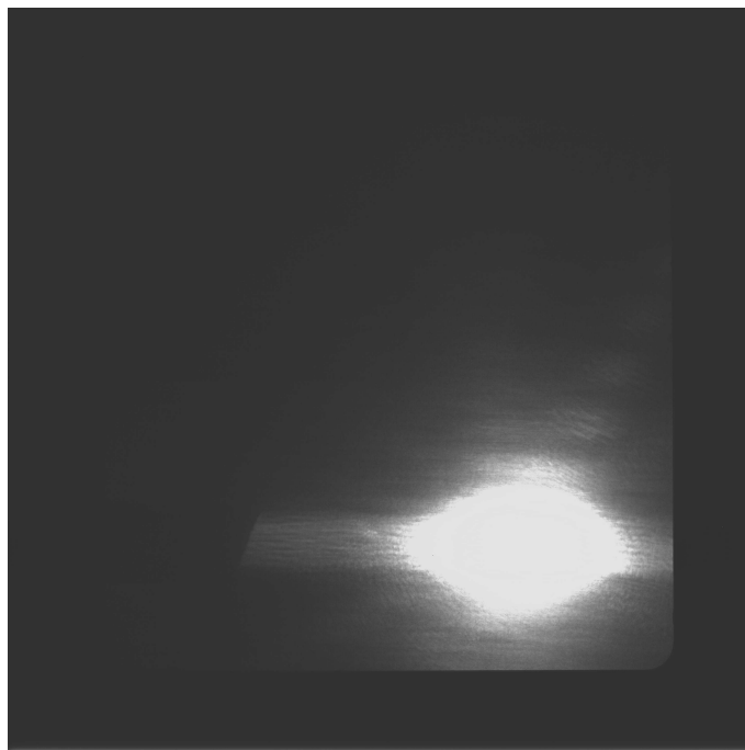
Fig. 17. HRI EUV first image acquired during ground calibration. Bottom right, the occultation of the EUV beam in the detector plane is visible.
